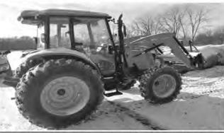
4609 Massey Ferguson Tractor w/DL 260 Joystick Loader 100 hp dual hydraulic 540 & 1000 PTO 1100hrs (diesel)
